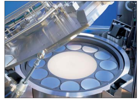
Aixtron's latest design uses either a 12 \times 4 inch or a 49 \times 2 inch configuration to deliver growth on substrates with a combined area of 150\text{ inch}^2 .
