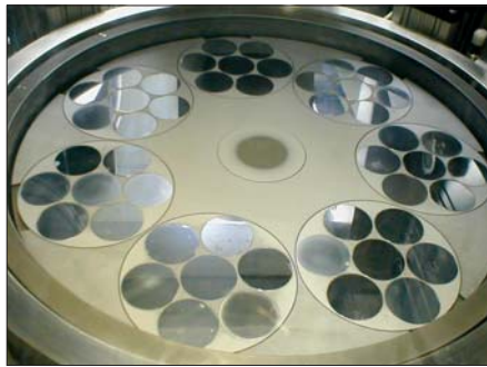
Aixtron's fully loaded 49 × 2 inch planetary reactor can produce epiwafers with uniformity suitable for LED manufacturing.
